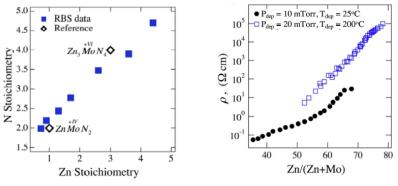
(Top): Theory predicts new stable  $Zn_3MoN_4$  and metastable  $ZnMoN_2$  in wurtzite-derived crystal structure. (Bottom): Experiments synthesize  $Zn_3MoN_4$ – $ZnMoN_2$  wurtzite alloys with composition-dependent electronic properties.
